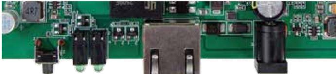
RESET INDICATORS SYSTEM POWER MOBILE WI-FI PoE & LAN DC SOCKET 9-48Volt
